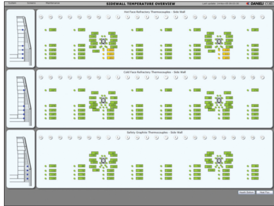
Fig 2 Overview of temperature display with alarm status for sidewall
